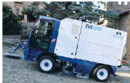
Sweeping and climbing over 20% full-load. The 4-wheel steering gives the M60 excellent manoeuvrability in all working conditions.
