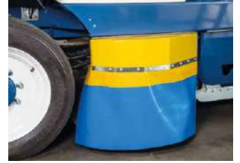
Side brush dust suppression skirts for dry dust-free sweeping.
