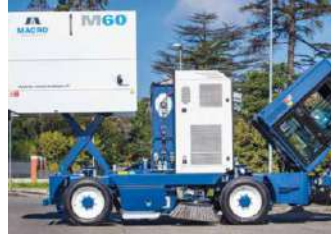
Dumping at any height between 1,1 and 2,3 m.
