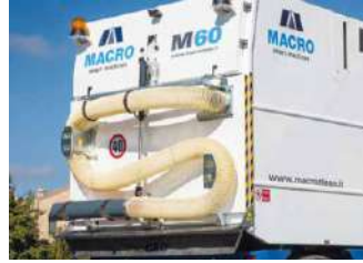
Rear powerful wandering vacuum hose, 6 m length -140 mm diameter.
