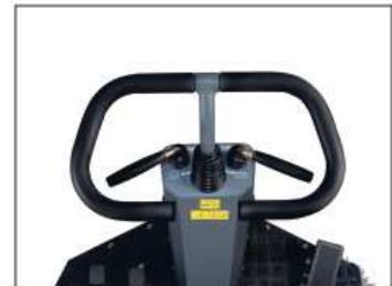
To facilitate effective and efficient cleaning operations, Brush controls are mounted on the steering column.
