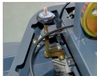
Easy access to broom adjustment system
