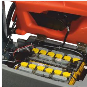
Large capacity battery pack
